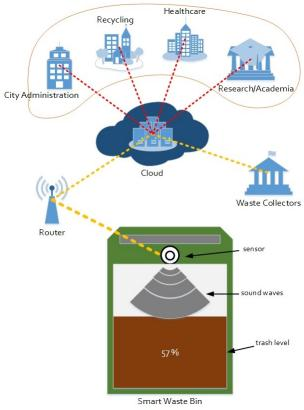
Figure 3. Cloud-based smart waste management architecture.
